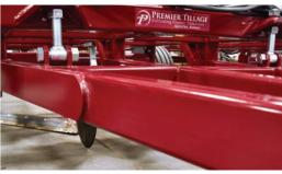
A longer, sturdier hitch with a redesigned center frame gives more turning clearance and greater level ability in the field.
