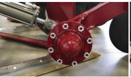
Our patent pending rock shaft system with rephrasing cylinders and internal spherical bearing for a no end play precision controlled leveling system.
