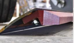
A 29-degree blade angle and thicker standard provides less flexing for higher ground speeds and greater vegetation kill.
