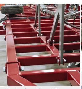
Front and rear hinge tubing made from 4x5 rectangular tube and designed to provide greater strength. All hinges have 1-1/4" grade 5 bolts.
