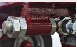
Adjustable bolt for performance leveling to your exact specifications, reducing fuel costs and making for a smoother pull.
